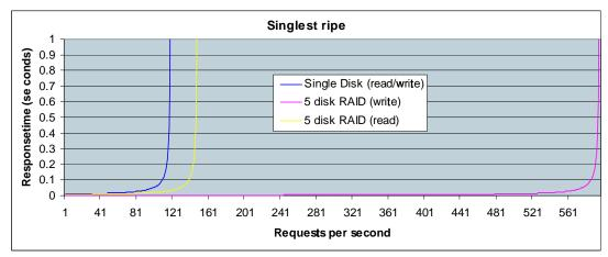
We see that in the case of single stripe reads, RAID 5 significantly outperforms a single disk. This is because the RAID configuration is able to exploit the parallelism between disks, exposing parallelism that does not exist in the single disk case. For writes, the RAID configuration also outperforms the single disk case, but by a much smaller margin.
