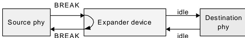
Case 2: OPEN address frame has propagated through the expander device:
